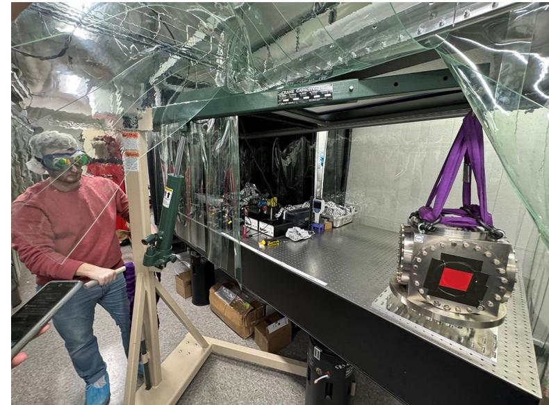
*Vacuum chamber used to hold mirror*
